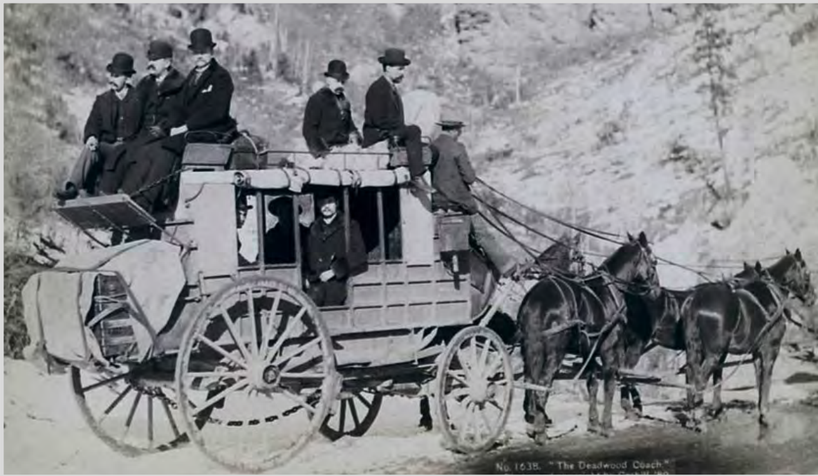
Above: A stage or celerity wagon of the Overland Mail Company (OMC). One hundred of the company's stage wagons were designed by Butterfield himself and were constructed by the James Gould Company of Albany, NY. The OMC used stage wagons rather than Concord coaches on 70% of the Southern Overland Route. Note that the number of passengers in the photo wasn't unusual, even for long trips.
