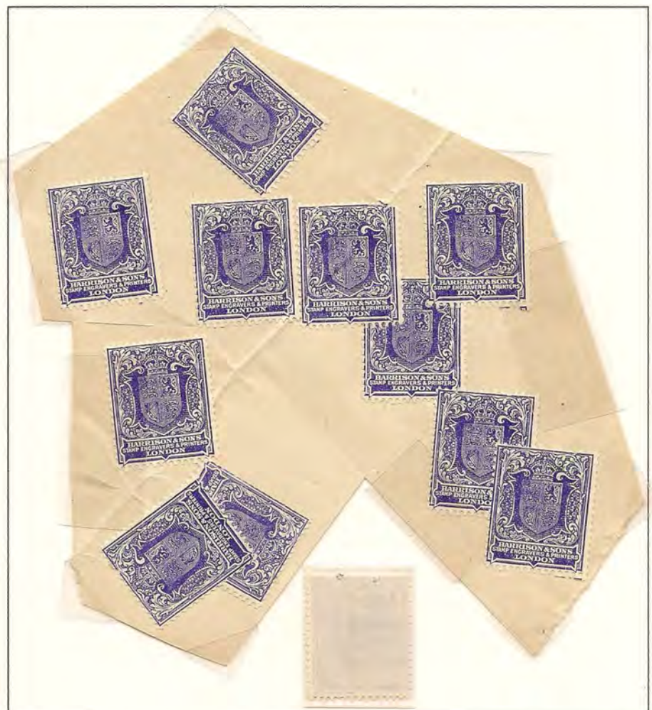
Test piece of eleven labels with two gripper marks and locating pin marks, as separate label shows. The Fixo stamp affixing machine applied these labels.
